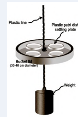
Figure 3. Diagram of the PICES collector used in this study (Valjejo, et al., 2017)
