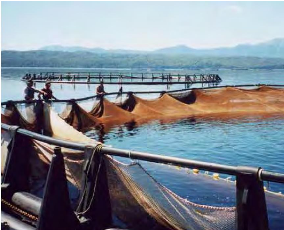
Photo 10 Net partly lifted for inspection
