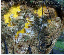
Waverider buoy deployed for >8 mths; fouling dominated by the barnacle Semibalanus balanoides .
