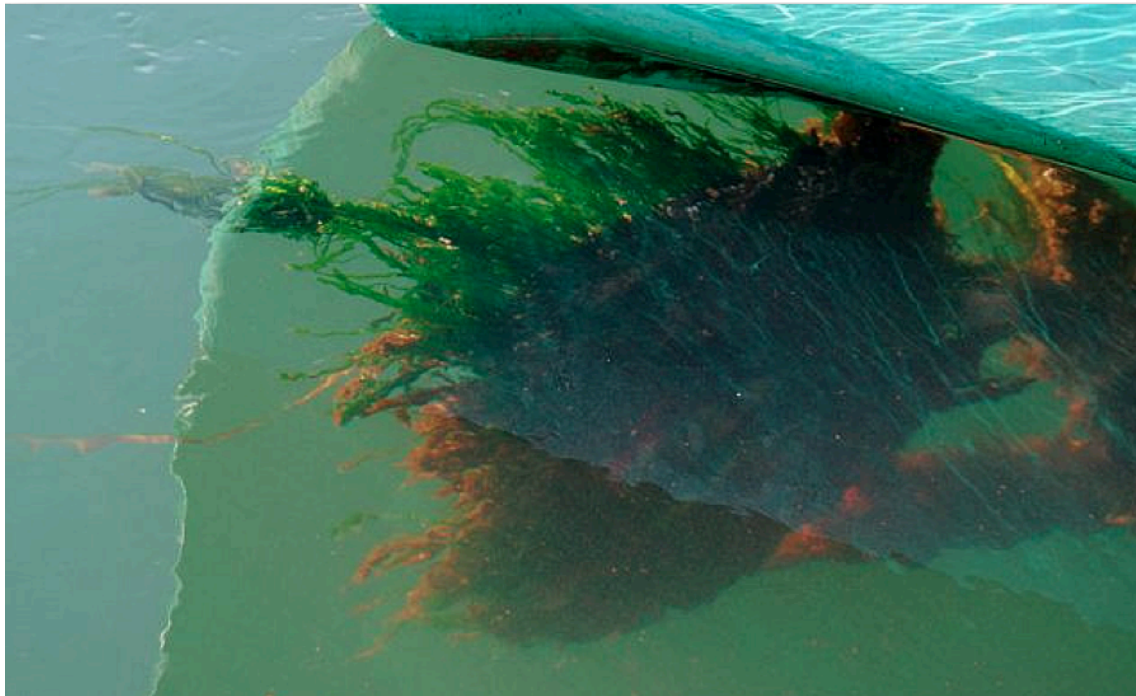
Figure 1. A boat rudder with a heavy cover of marine biofouling (photo: B.A.P. da Gama)
