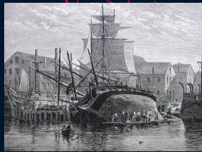
Careening of a ship - An Old Whaler Hove Down For Repairs, Near New Bedford, a wood engraving drawn by F. S. Cozzens and published in Harper's Weekly, December 1882.
