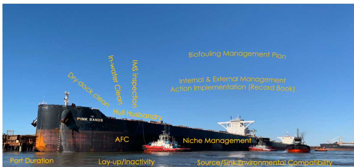
Figure 2: Vessel-Check metrics used to assess the management practices employed by a vessel to mitigate the transfer of invasive aquatic species to as low as reasonably practicable
